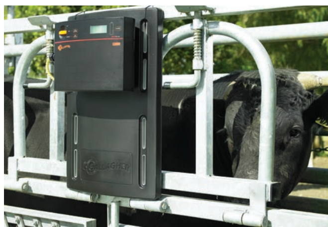
The BR reader automatically reads the animal's tag as soon as the animal is in the crate.
