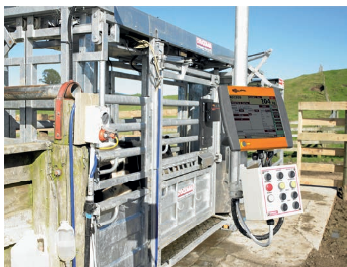
The TS2 weighs livestock and collects data for improved livestock management
