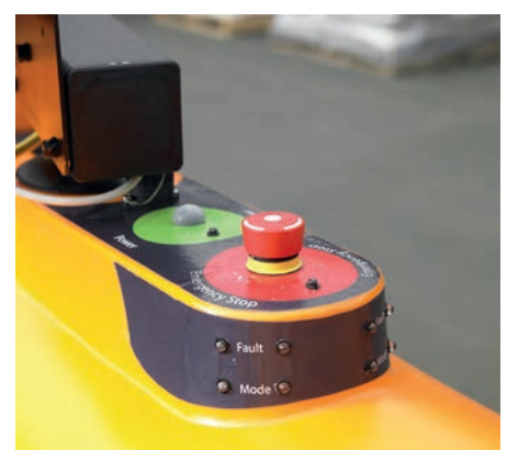
High visibility control panel - Includes emergency stop button, auto/manual status & fault lamp.
